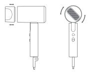
CAUTION: To avoid burns, do not adjust, install, or remove the air nozzle during use.
